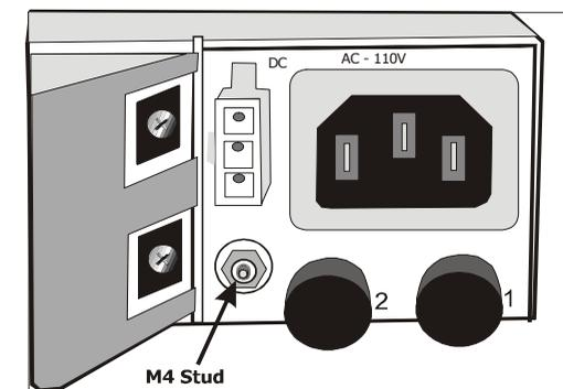
Use an M4 nut and M4 lock washers with the parts stacked as shown in the figure below.
